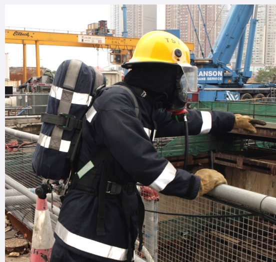
● 新呼吸器可即時由單瓶轉為雙瓶模式運作，適合處理隧道事故 New BA can change from single-cylinder to twin-cylinder set up instantly which is suitable for tunnel incident
