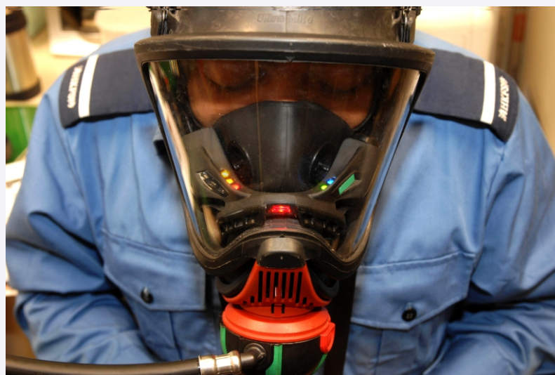
● 面罩內設抬頭顯示器顯示氣樽存氣量及撤離警告等訊息 The Heads-Up Display inside the facemask indicates cylinder pressure and withdrawal signals to the BA wearer
